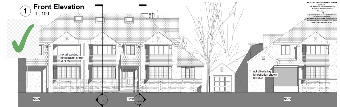
Above No31 as planning approval 2021 – only the side dormer windows steps down from the existing ridge line.
