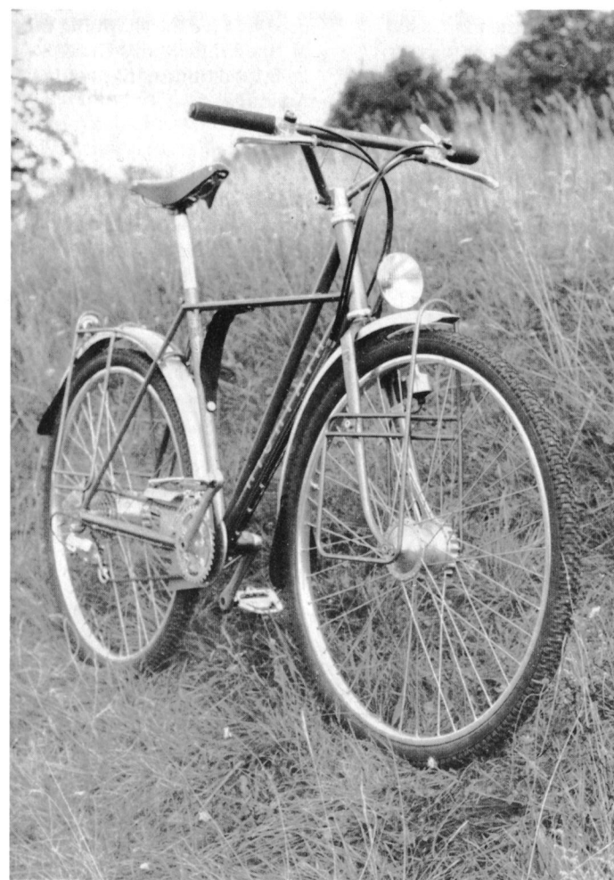
Above: an experimental suspension bike. Left: a £2,000 28" wheel tourer with cro-mo racks, lighting, and 21 gears. All photographs by David Wrath-Sharman unless otherwise credited.
